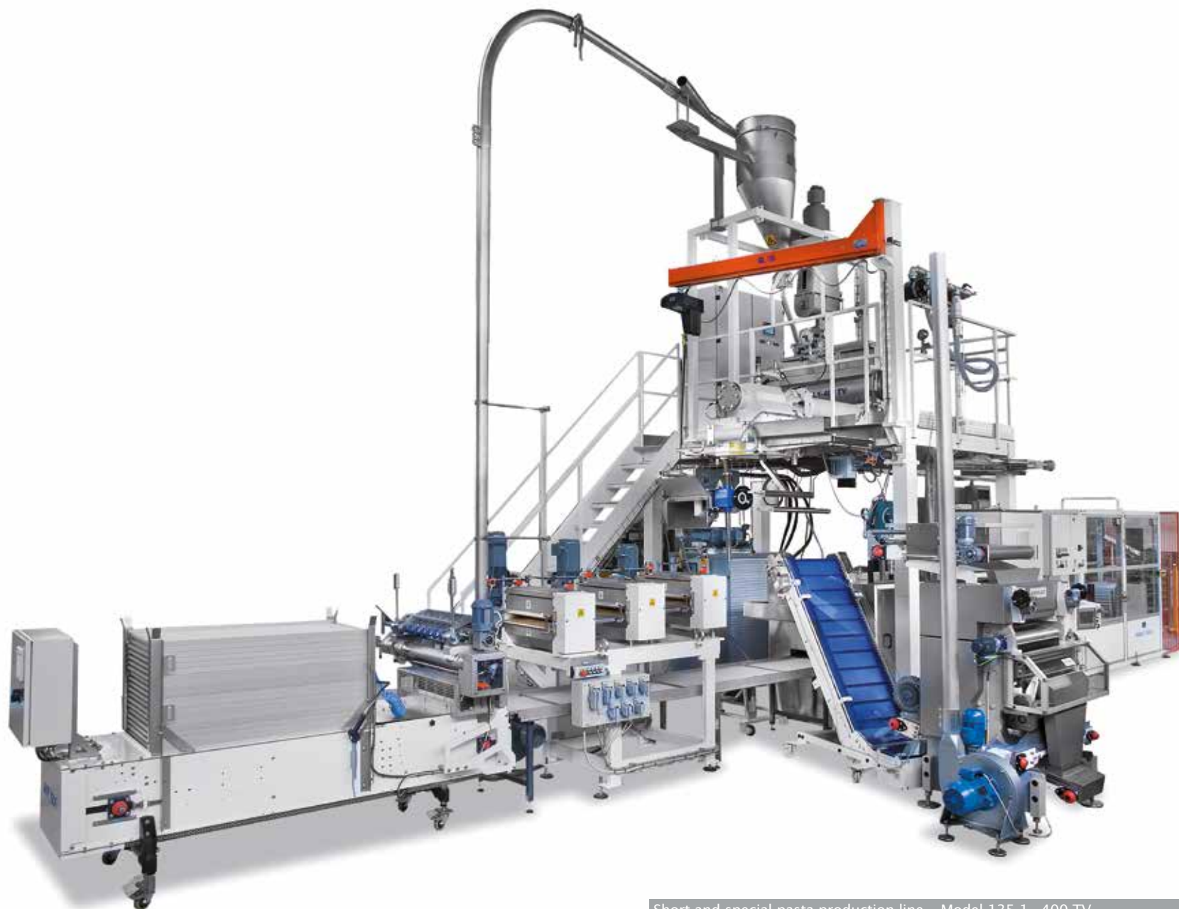
Short and special pasta production line – Model 135.1- 400 TV
