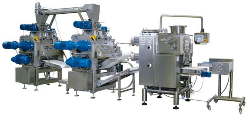
STF-540TV DOUGH SHEETERS AND RCA540-B RAVIOLI MAKER
