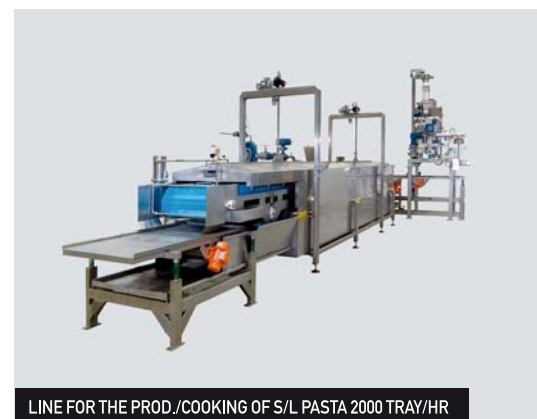
LINE FOR THE PROD./COOKING OF S/L PASTA 2000 TRAY/HR
